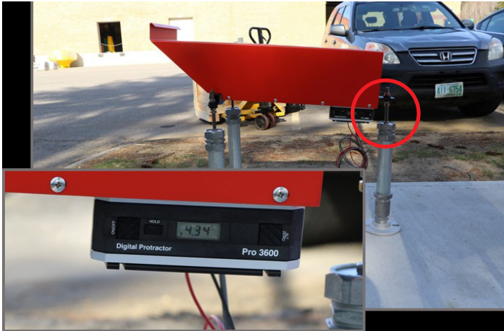
Inclinometer Positioned On Top Of The Inclinometer Bracket
