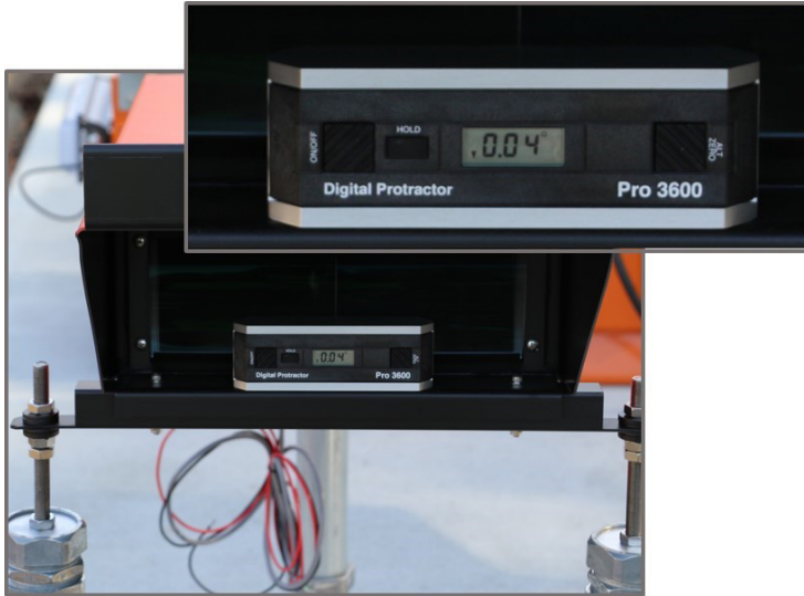
Inclinometer positioned in the middle of the front of the base plate
