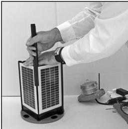
5. Slide the rubber corner out of the chassis, it may be necessary to lubricate the edges of the solar panels with grease or oil based lubricant if this is difficult to remove.
