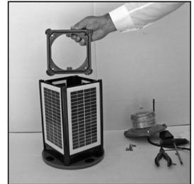
4. Remove 4 x M6-35mm long socket head cap screws, to remove the top casting from the chassis.
