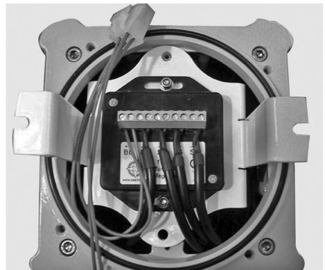
SL10 AMP Regulator shown when correctly fitted
