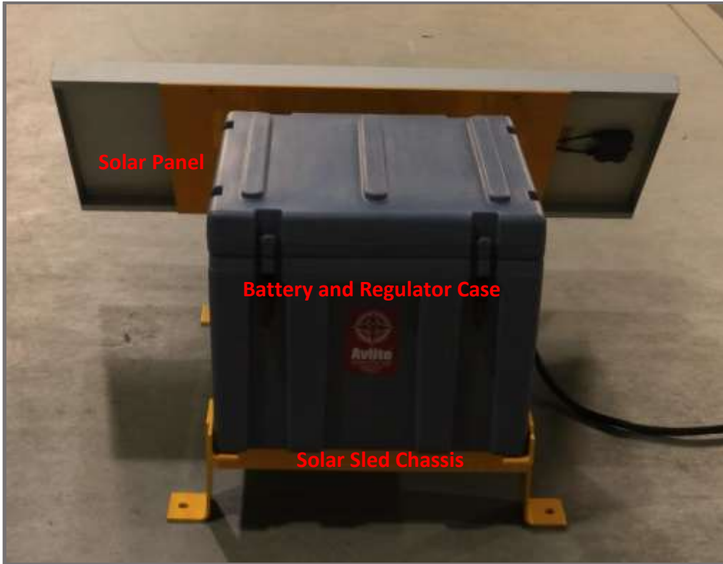
Figure 6: Solar Panel and Components Rear View
