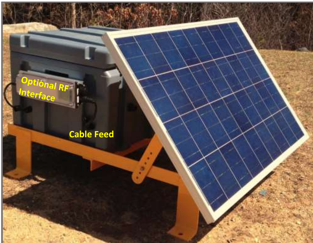
Figure 7: Solar Panel and Components Side View
