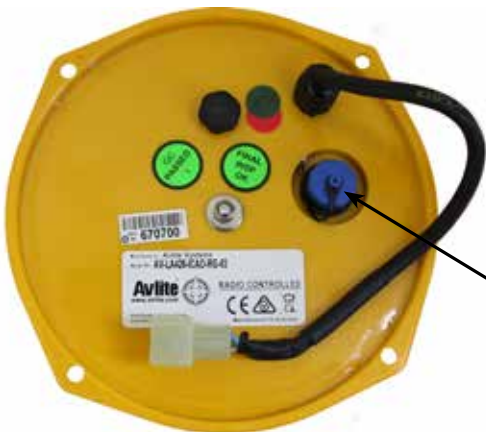
Programming Port Replace blue cap after programming
