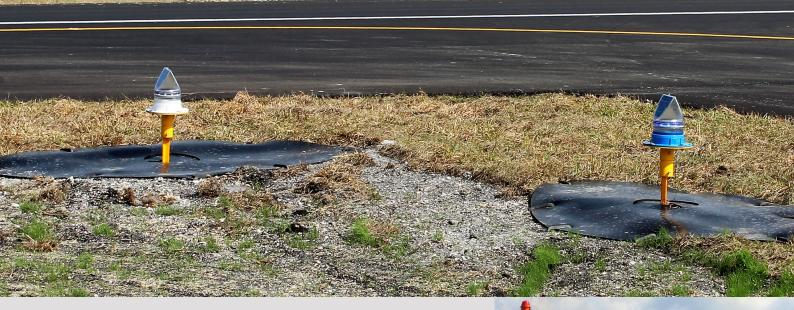
**Above:** Avlite's AV-70 White (runway) and AV-70 Blue (taxiway) are compact solar aviation lights. Completely self-contained, each light features two high performance solar panels within the lens to maximize solar collection, and a user-replaceable battery. Made from durable, UV stabilized LEXAN® polycarbonate and incorporating an internal photodiode for automatic night activation once the ambient light threshold drops, the AV-70 can be installed in moments.
