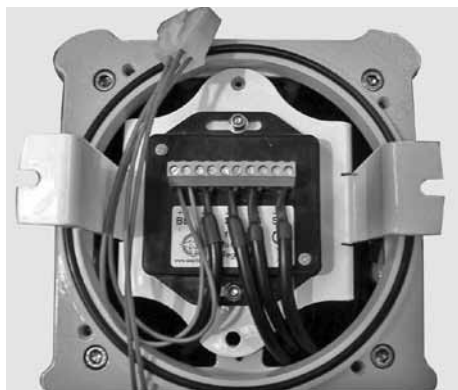
SL10 AMP Regulator shown when correctly fitted
