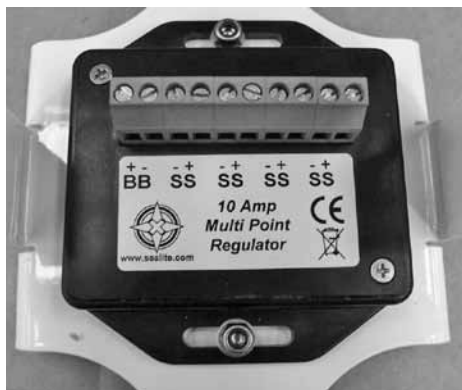
Use the label to ensure correct location of wires during assembly
