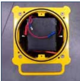
1. Remove 4 x socket head cap screws and disconnect the light head from the chassis.
