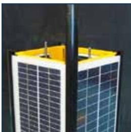
6. Slide the rubber corner out of the chassis. It may be necessary to lubricate the edges of the solar panels with grease or oil based lubricant if this is difficult to remove.
